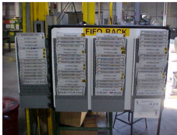
FIFO (first-in-first-out) Rack at heat treat.
